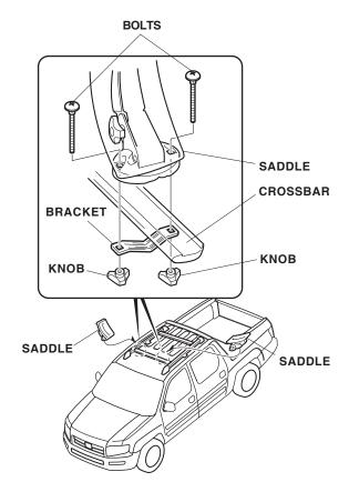
Position the two hydro-glide assemblies on the rear crossbar. Loosely install the hydro-glide assemblies using one bracket, two bolts, and two knobs for each assembly. The distance between the two assemblies should be the same as the width of the kayak.
