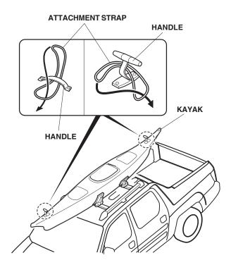
12. Attach one ratchet hook to the front attachment strap and one ratchet hook to the rear attachment strap. Attach the front hook to the front bumper beam or to the tow hook. Attach the rear hook to the rear tie-down anchor in the bed. Secure the kayak to the vehicle by pulling the ropes through the ratchet hooks.
