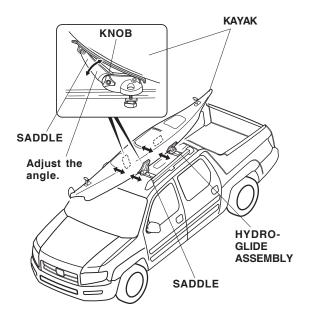
Slide the kayak forward or backward until it's level with the roof. If necessary, loosen the knob on each saddle and adjust the saddle angle to fit snugly against the kayak. Tighten each knob securely. 6. Route each strap with buckle through the buckle cover with the ribbed side facing up as shown.
