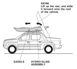
4. Adjust the distance between the saddles and hydro-glide assemblies to the same width as the kayak, then secure the saddle and the hydro-glide assemblies by tightening the knobs you installed in steps 1 and 2.
